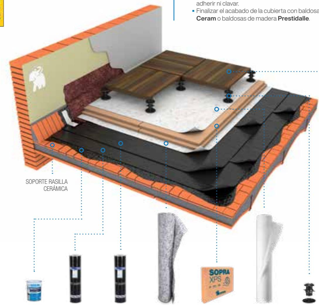
Emufal Primer Elastophene Elite FV 4 kg Sopralene Elite FP 4 kg Rooftex V 200 SopraXPS SL 80 Texxam 1000 Soportes Regulables Suprema Sopradalle Ceram
